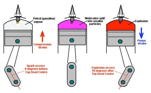
Because of the delay needed for the conversion of the hydrocarbon molecules to smaller particles, the spark is arranged to occur before the Top Dead Centre point. While the molecules are splitting up, the piston passes its highest point and the crankshaft is some degrees **past** Top Dead Centre before the driving pressure is placed on the head of the piston. This driving force then reinforces the clockwise rotation of the crankshaft shown in the diagram above and the motor runs smoothly.
